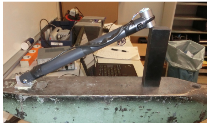
Figure 2: Test rig for accelerometer mounting evaluation
