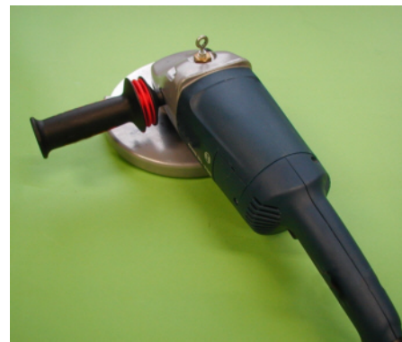
Schematic diagram showing the vibrating structure (top) vibration-attenuated auxiliary handle on an angle grinder (below)
