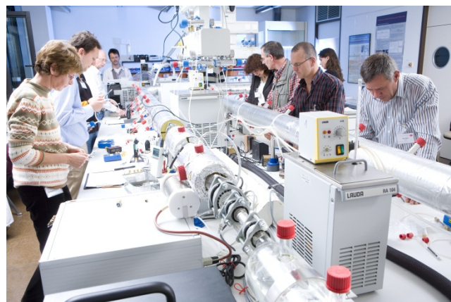
Test gas stream for the performance of round-robin tests including sampling at the IFA
