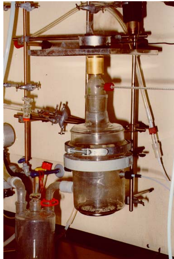
Apparatus for study of the flammability behaviour of respiratory filters
