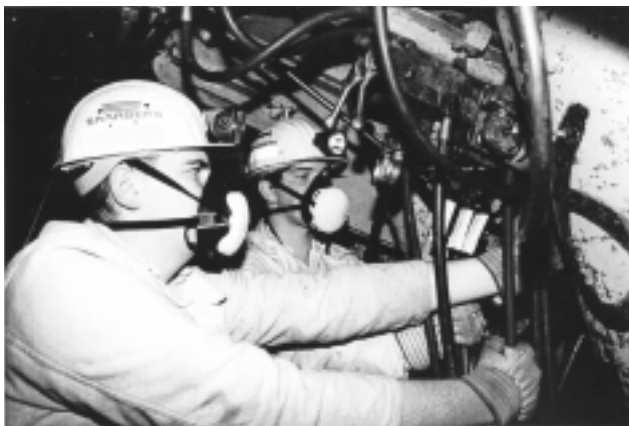
Figure 6: Filtering dust protection mask, type Picco 20 SA, used in underground mining
